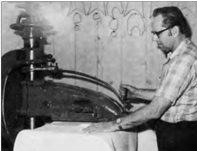
Jens Sorensen operating the factory's "stamper" machine in 1973. By pressing down with great force on a steel die the stamper cut leather used for the top part of the wooden shoes. Different shapes of dies can be seen hanging on the wall behind Jens. Photo used with the permission of The Danish Villages Voice.
